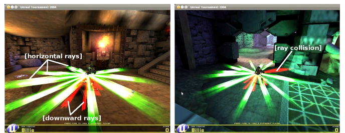
Fig. 4. Backup navigation based on ray casting
